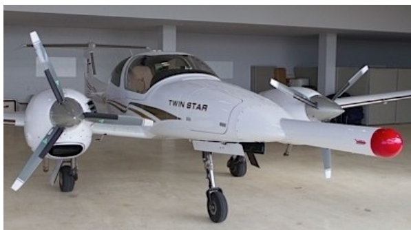
TOTEM-2A VLF Nose Stinger (Photo courtesy of Tundra Airborne Surveys Ltd.)
